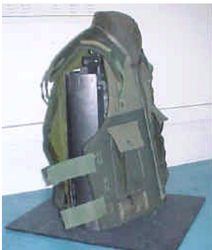
Goldorac II, an adjustable torso mechanism employed in body armour testing
